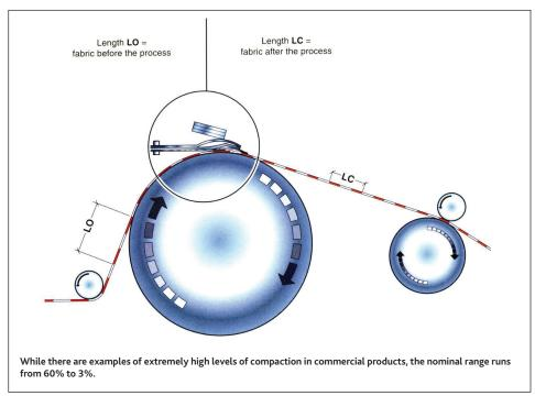
How does this relate to elongation? Depending upon a number of process variables as well as the nature of the compacted sheet, some or all of the compaction can manifest itself as elongation. A material compacted 50% can then represent 100% elongation.
